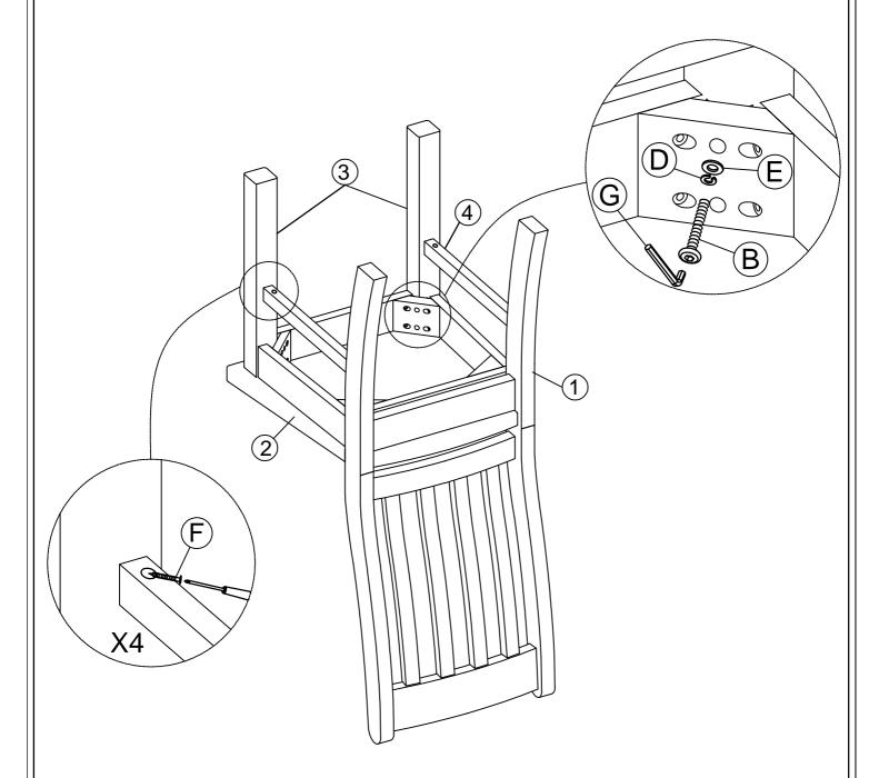
"Important Note - Before finally tightening the bolts, place the assembled chair upright on a level surface and sit carefully on the chair to ensure the chair legs are aligned and level. Then fully tighten all bolts and your chair is ready for use."
